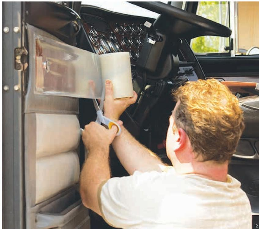
During manufacturing and transport, transparent 3M™ Polyethylene Protective Tapes protect many finished automotive interior surfaces from abrasion, nicks, and scratches. Clear acrylic adhesive holds with very low tack for easy removal.
