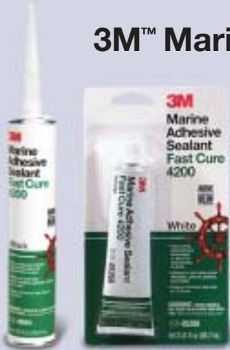
A one-part, general all-purpose polyurethane that chemically reacts with moisture to deliver flexible bonds with good adhesion to wood, fiberglass, gelcoat, plastics and metals. Forms watertight, weather-resistant seals on
