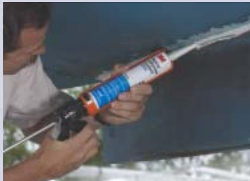
This high-performance polyurethane adhesive sealant becomes tack-free in 24-48 hours, and completely cures in 5-7 days with no shrinking. The seal is extremely strong, retaining its strength above or below the waterline. Stays flexible—allows for structural movement. Stress caused by shock, vibration, swelling or shrinking is effectively absorbed. Has excellent resistance to weathering and salt water. Check the bonding and sealing jobs this product can handle for you:
