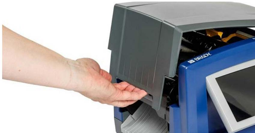
2. Release the latch on the ribbon cover [2] and swing open.
