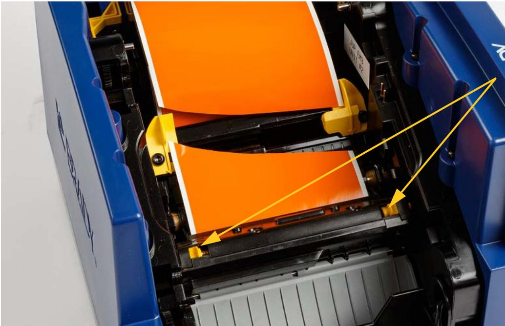
3. Rotate the cutter gear counter-clockwise to lower the blade.
