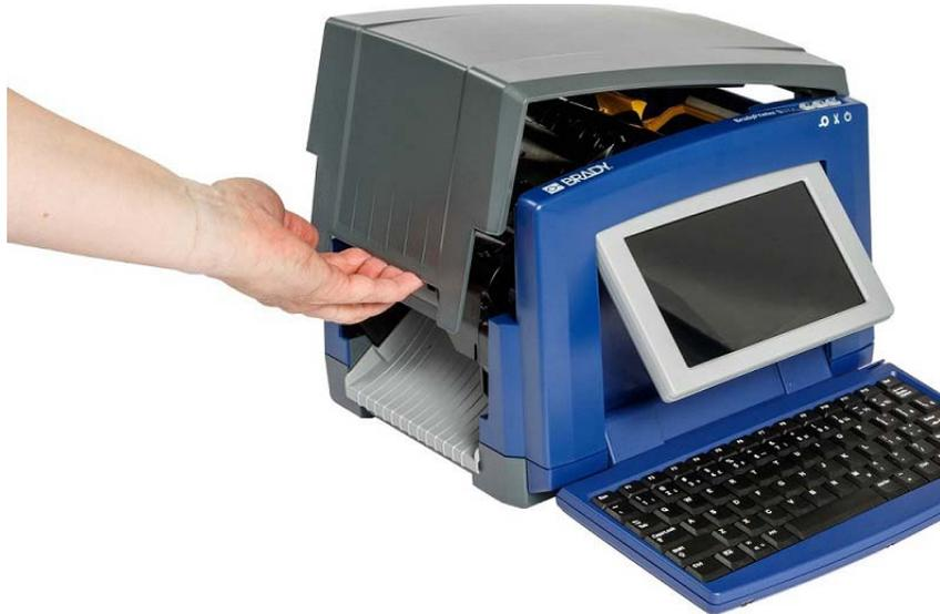
2. Release the latch on the ribbon-cover [2] and swing open.
