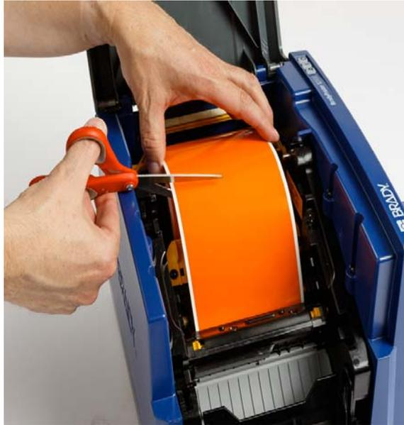
2. Squeeze the tabs to release and tilt the cutter module.
