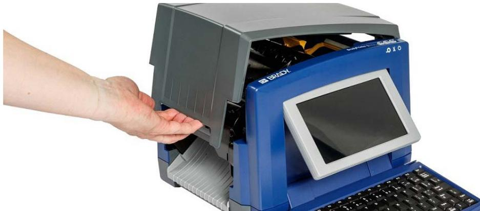
3. Release the latch on the ribbon cover [2] and swing open.
