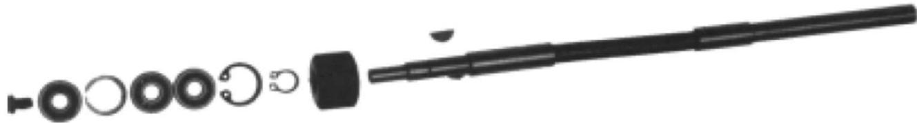
11. Remove button head screw 625068 to release spindle bearings 863582 and shims. Remove retainer ring 833774 to release spindle gear 622097 and key 622057.
