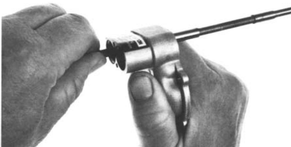
8. Remove the spindle adjustment screw 625026 by screwing the spindle clockwise through the backhead assembly 625020.
