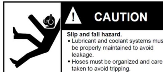
10QNP drills can be used with lubricant or cooling systems which must be properly maintained to avoid leakage. Failure to do so can result in serious injuries from slipping on oily surfaces.
