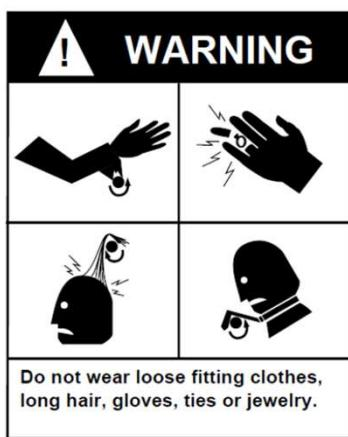
Follow good machine shop practices. Rotating shafts and moving components entangle and entrap, and may result in serious injuries. Never wear long hair, loose-fitting clothes, gloves, ties, or jewelry when working with or near a drill of any type.
