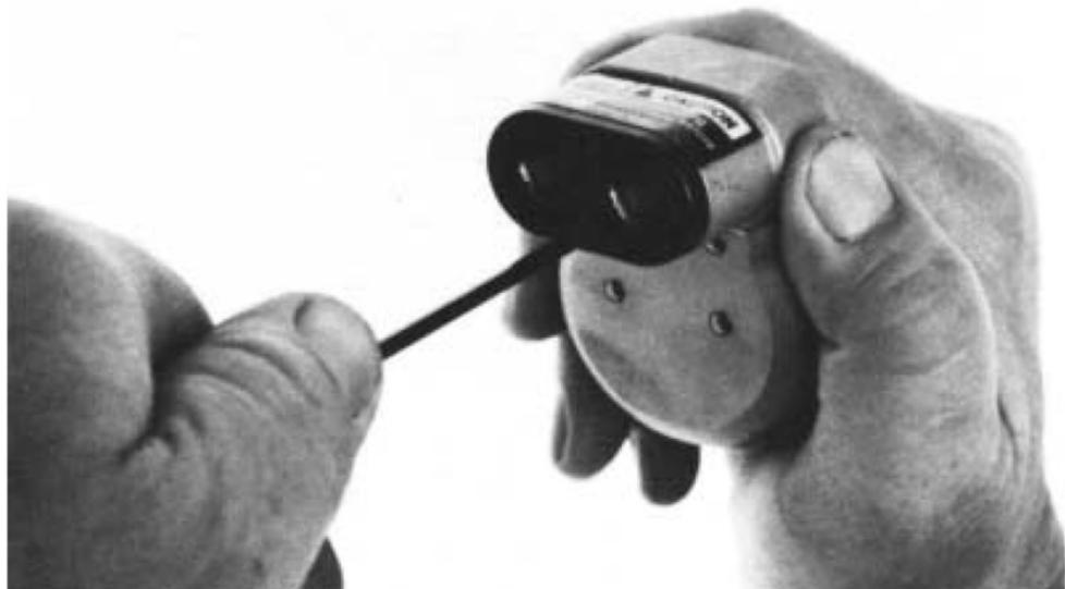
9. Remove two socket head cap screws 622774 from spindle adjustment plate 625019 and remove plate.
