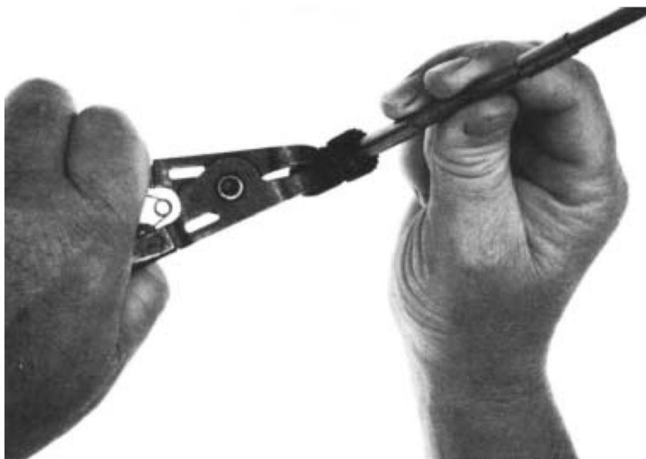
10. Remove retainer ring 623685 with bent internal pliers. Pull off spindle adjustment screw 625026 to expose bearings.
