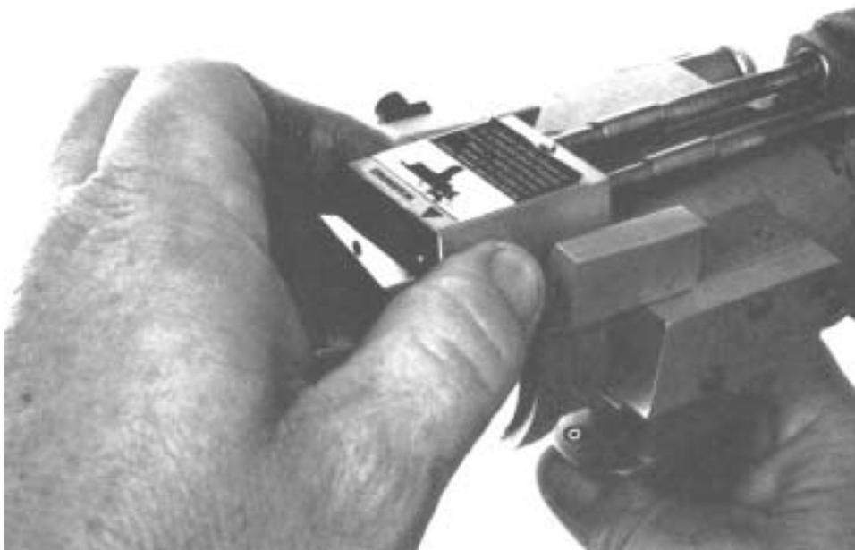
3. Remove support plate from spindles.
