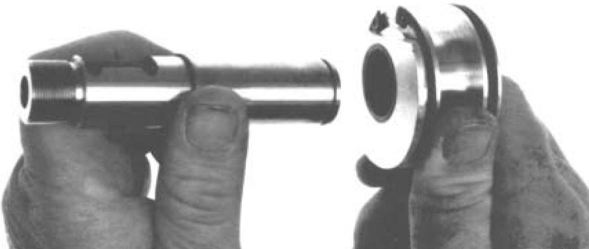
2. Remove clamp feed shaft spiral ring 623595 and slide clamp feed shaft 625030 out of front enclosure 625029.
