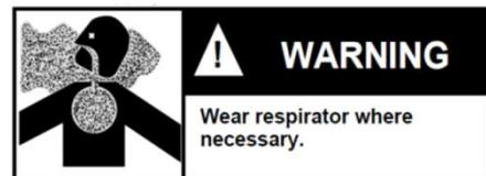
Drilling or other use of this tool may produce hazardous fumes and/or dust. To avoid adverse health effects, utilize adequate ventilation and/or a respirator. Read the material safety data sheet of any cutting fluids or materials involved in the drilling process.
