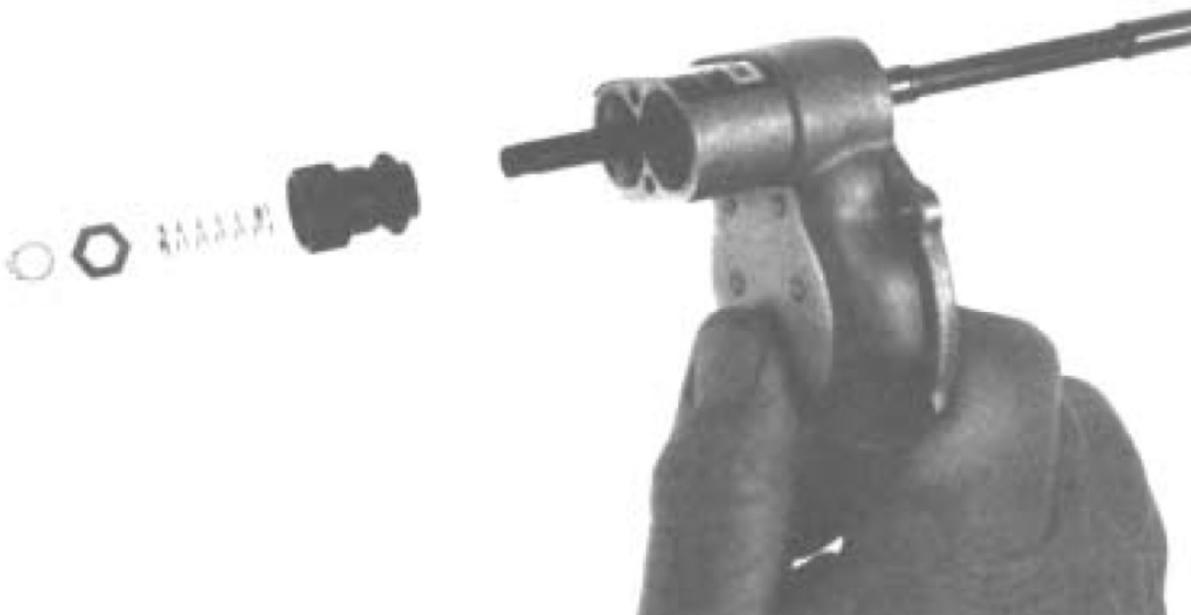
7. Remove retainer ring 625467 to release spindle adjustment nut 625027, adjustment knob spring 622140 and adjustment knob 625023.
