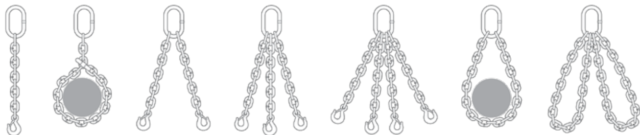
SINGLE LEG (VERTICAL) SINGLE LEG (CHOKER) DOUBLE (2 LEGS) TRIPLE (3 LEGS) QUADRUPLE (4 LEGS) BASKET TYPE DOUBLE BASKET TYPE
