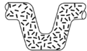
CASTING Random grain flow with larger grain structure makes material weaker than forged products
