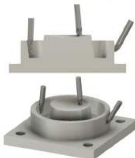
The images above show the comparison of a ball end mill to an oval shape Multi-Axis Finisher with a benefit multiple of 8.
