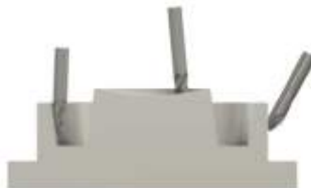
The images above show the comparison of a ball end mill to an oval shape Multi-Axis Finisher with a benefit multiple of 4.
