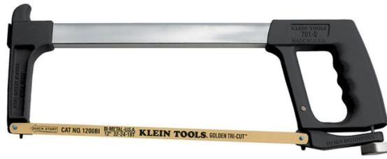
This versatile hack saw blade has three teeth sizes and the ability to quickly convert the blade to 90- or 45-degrees for standard or flush-cut applications. The Pivot-lock adjusts blade tension for straighter cuts and longer blade life. It also features a set screw which allows for storage of extra blades and secures blade for "jab" sawing.
