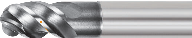
4 flutes, Helix angle 45° Dedicated carbide substrate gives excellent wear resistance.
