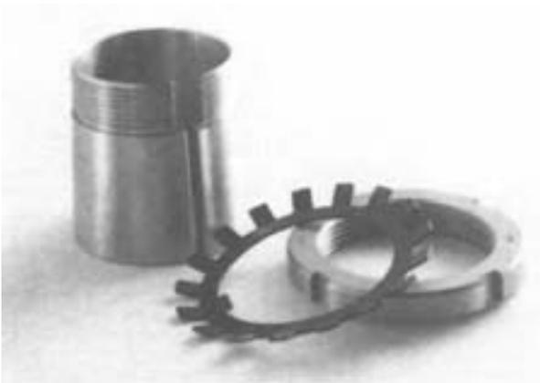
The Lockwasher with the straight inner tab must be used with the narrow slot type of adapter sleeve (suffix X)
