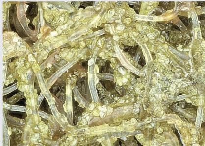
*Flexible, non-woven construction with high concentration of active mineral sites for fast, consistent cutting without compromising final finish. Specially coated to minimize loading. Produces controlled, uniform scratch throughout life of the abrasive.*
