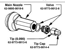
3. Remove warmed cartridge and insert main nozzle assembly into the Bench Wrench. The front of the applicator can be used if a Bench Wrench is not available.
