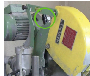
Example of easily mounting a Bat Nozzle to a circular saw.
