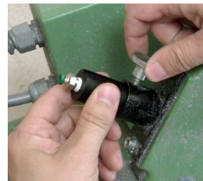
Example of easily mounting a Bat Nozzle to a circular saw.
